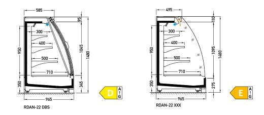
**DBS** – door | double, bent | sliding (sideways) **XXX** – no glazing
